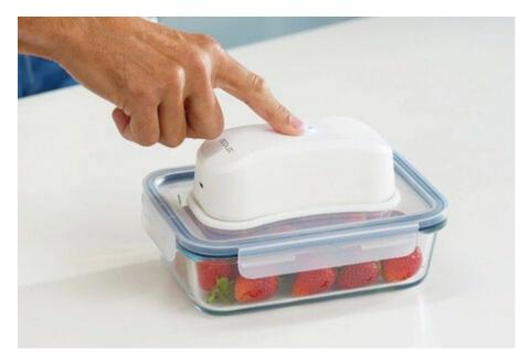
Instead, the chip leverages a physical process called cathodoluminescence to emit primarily UVC light, along with some UVA and UVB light, when excited by electrons. It's designed to initially turn on for a few minutes when food is placed in the container and then automatically turn off using a built-in timer. Users can then choose to turn it on for a few minutes each day.
